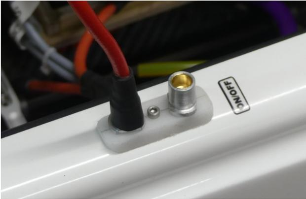
*Fig.7 A safety loop provides an essential way of disconnecting the power between the motor and the battery. Here a connector is supported in an aluminium holder and a nylon support, the gold-plated connector provides the best electrical contact and therefore least power loss.*
