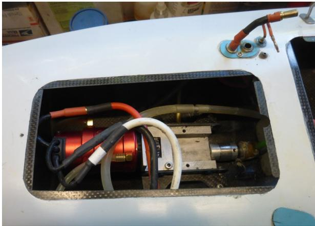
*Fig.1 A neat installation to convert a geared multi-boat to an electric racer, note the safety loop and external ESC arming arrangement*
