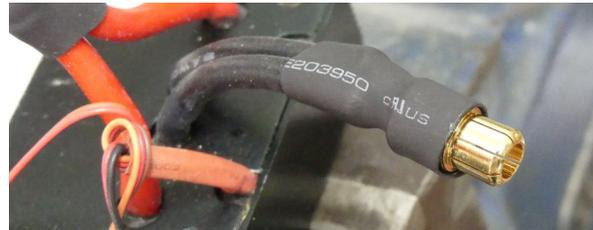
*Fig.6 Heat shrink to support the joint and 10 mm male connector*
