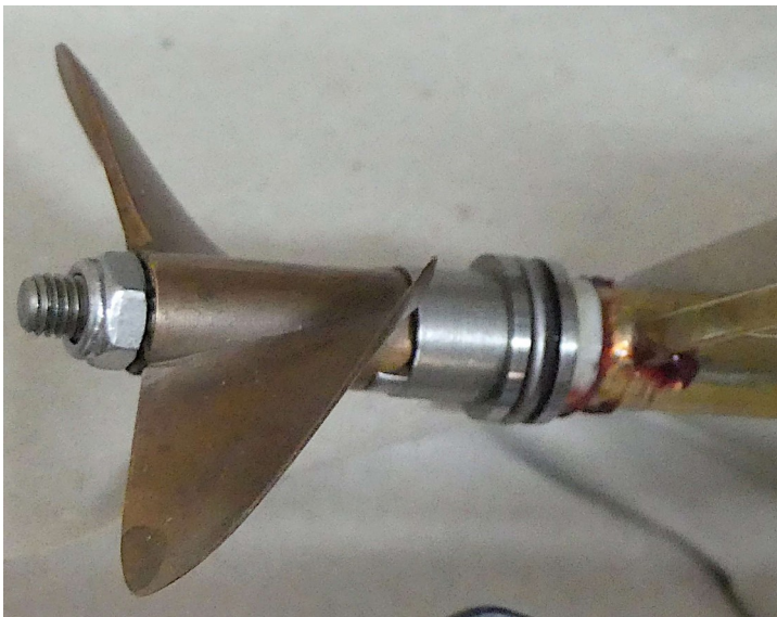
Photo illustrates a thrust race between the shaft dog and a nylon washer. ©GNP
