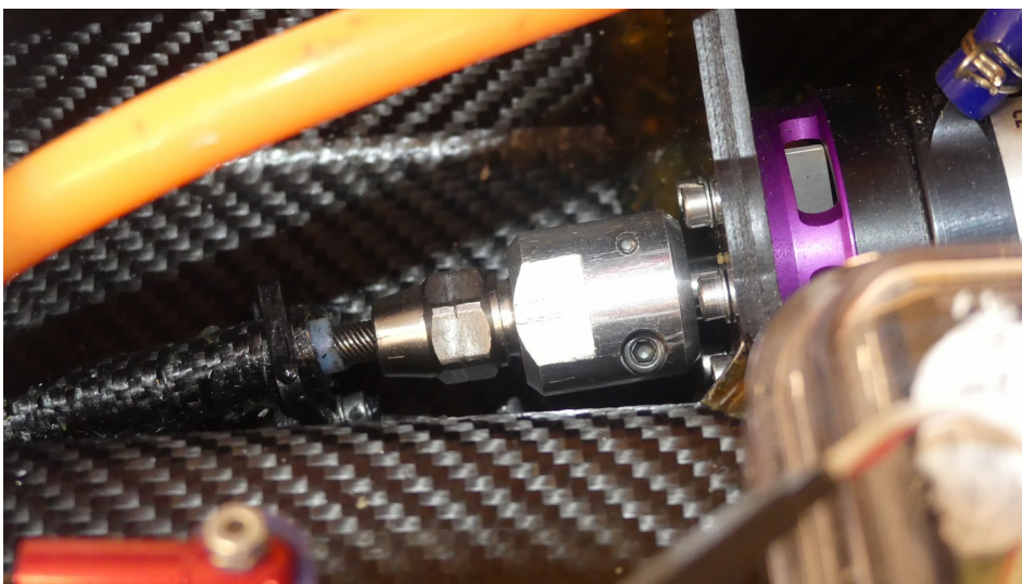
Photo of an Lehner motor closely coupled with a 5 mm diameter flexi-shaft aligned in the construction phase. ©GNP
