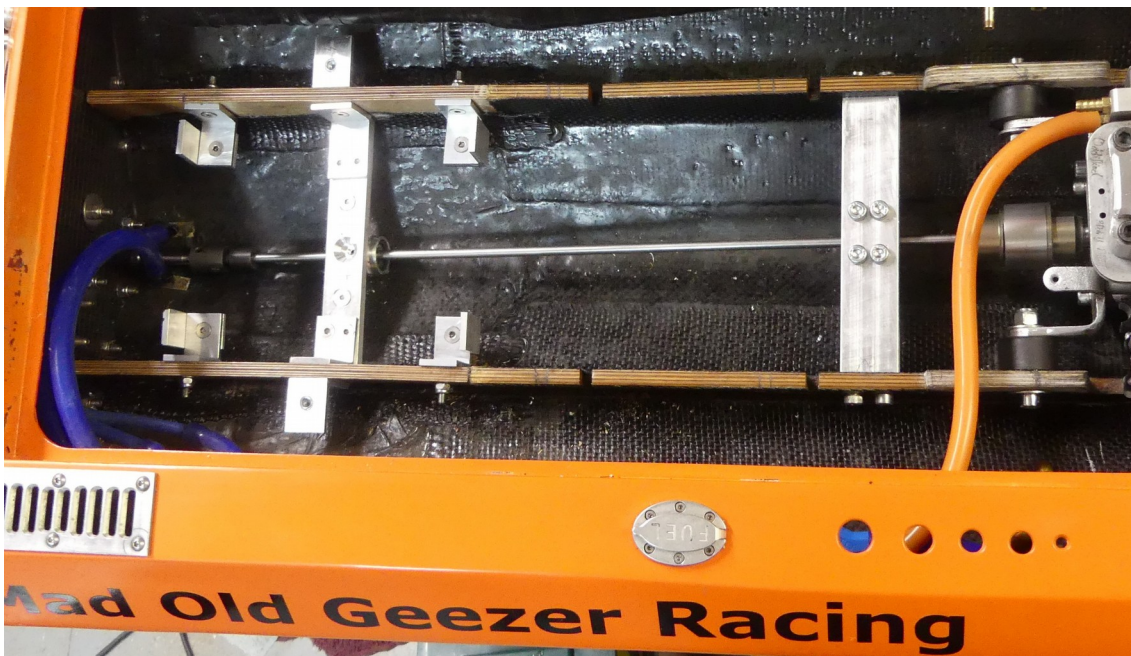
Photo of a solid 5 mm diameter shaft installation using a single ball-and-socket joint at the stinger end and a Kalistratov coupling at the engine end. ©GNP
