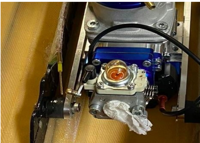
Fig.2 An SG27 motor with a cable and ball-joint connection to the throttle.
